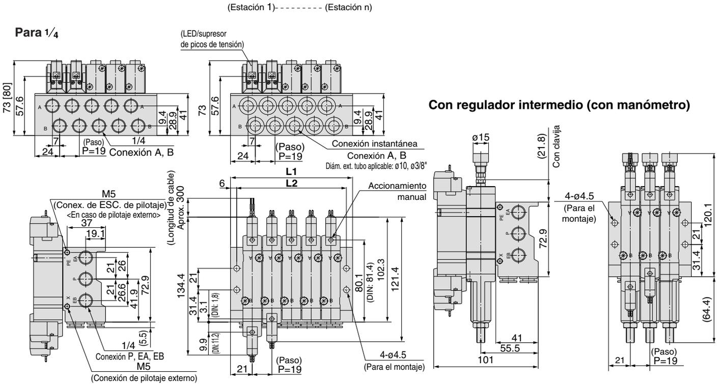
Conector enchufable L (L) Conector enchufable M (M) Conector DIN (D) Conector M8 (WO)
