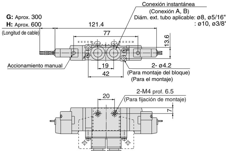
Conector enchufable L (L): SY7220-□<sub>L</sub>□<sub>C8, N9</sub>□<sub>C10, N11</sub>□(-F2)-Q
