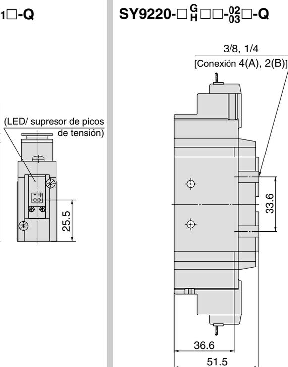
Conector enchufable L (L): SY9220-□L□□-<sup>C8, N9</sup><sub>C10, N11</sub>□-Q
