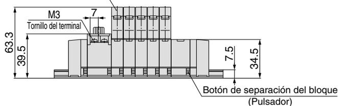
Equivalente al multiconector sub-D aplicable {JIS-X-5101, MIL-C-24308}
