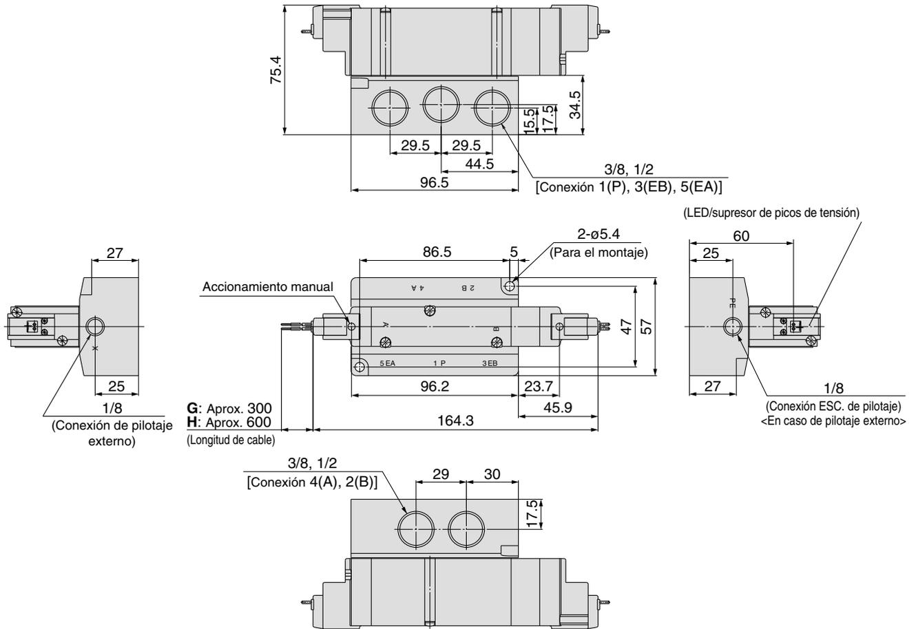
Conector enchufable L (L): SY9<sup>3</sup>/<sub>4</sub>40(R)-□L□□-<sup>03</sup>/<sub>04</sub>□-Q
