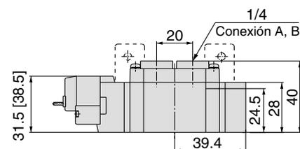
Conector enchufable L (L): SY7120-□L□□-C<sub>8, N9</sub>/<sub>C10, N11</sub>□(-F<sub>2</sub>)-Q
