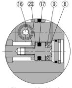
Rod cover Piston rod B-side piston
