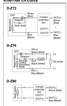
Note) A contact protection box should be used in any of the following conditions to prevent the shortening of the working life of the switch. (Refer to page 40 regarding the detailed specification for contact protection
