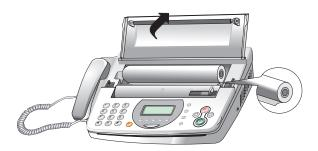
**2** Place the front edge of the paper into the paper guide. Pull the paper forwards, until the panel is covered.
