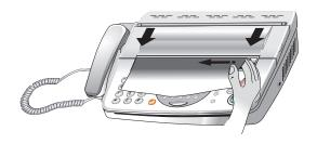
If a red line appears on the printout, the paper supply is almost over. Insert a new paper roll into the device.
